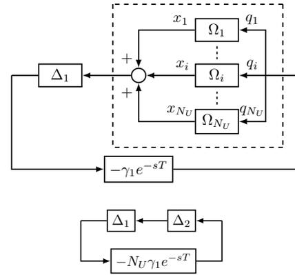
Fig. 3. Simplified network with one link and  $N_U$  users with round trip time  $T$  for each user. Stability is tested on the two system interconnection.
