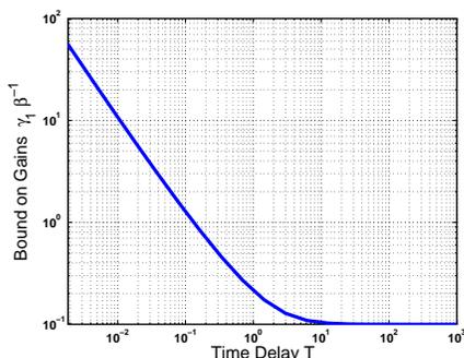
Fig. 4. Robustness test for the Internet congestion control problem with a static link (25) and dynamic user algorithm in (23) with  $N_U = 10$ . The bound on the gain  $\gamma_1\beta^{-1} \rightarrow \frac{1}{N_U}$  as the time delay  $T \rightarrow \infty$ .
